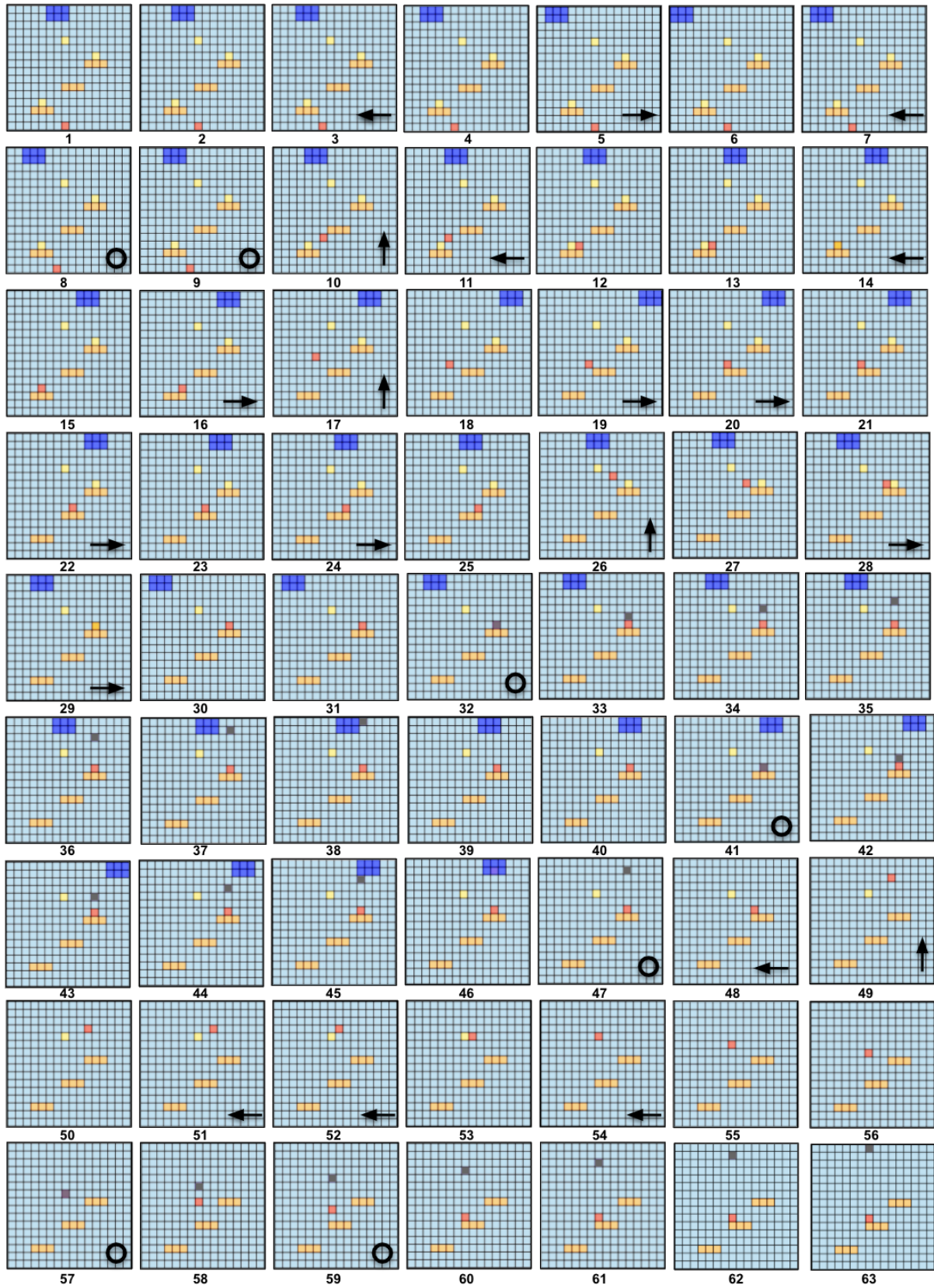
Figure 6. A full observation trace from the Mario program. Black arrows indicate user keypresses and circles indicate user clicks.
